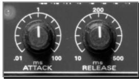
Attack sets the speed at which the compressor 'acts' on the input signal. A slow attack time (fully clockwise) allows the beginning envelope of a signal (commonly referred to as the initial *transient*) to pass through the compressor uncompressed, whereas a fast attack time (fully counter-clockwise) immediately subjects the signal to the ratio and threshold settings of the compressor.
